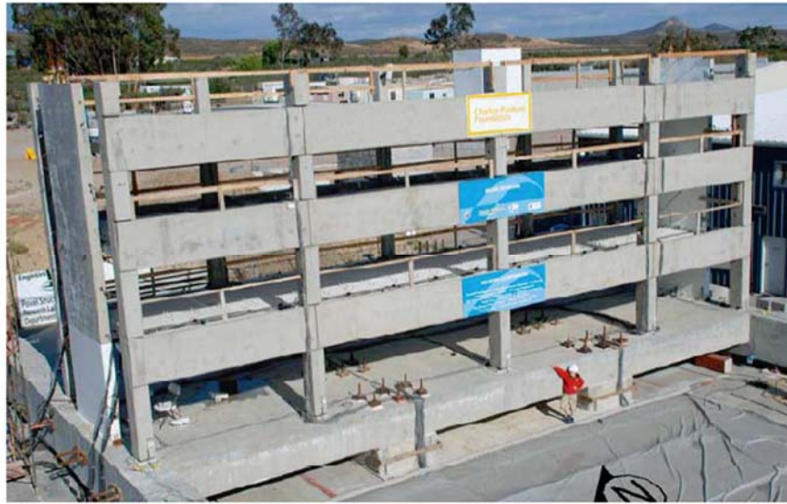
Figure 2-19. Shake table test of precast concrete building at UCSD (Fleischman et al. 2005)
